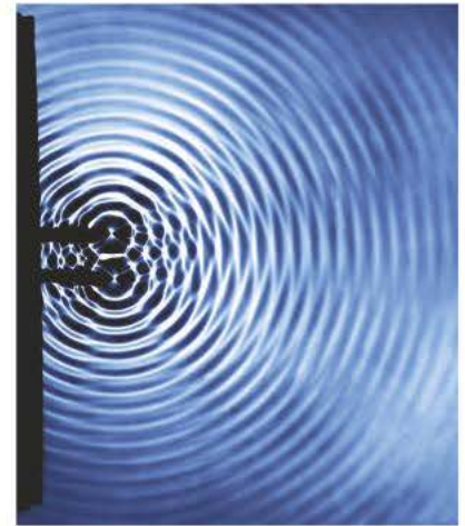
▲ Figure 3 Interference of water waves
