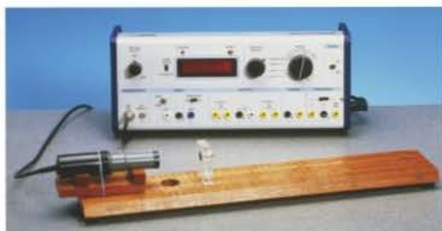
a a Geiger–Müller tube connected to a scaler counter
