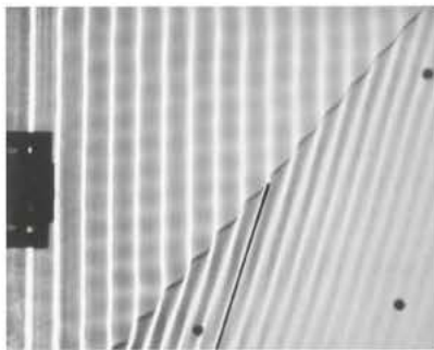
▲ Figure 2 Reflection of plane waves
