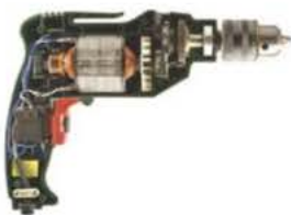
▲ Figure 8 A practical electric motor
