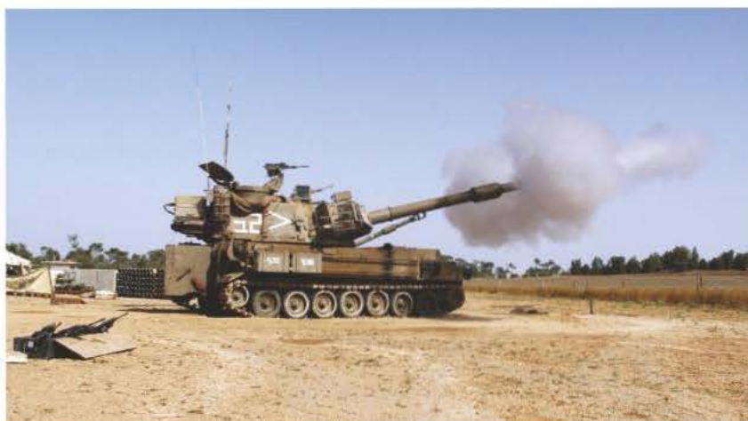
▲ Figure 1 The gun barrel recoils when the shell is fired. Large springs fitted to the barrel take away and store the kinetic energy of the barrel as it recoils
