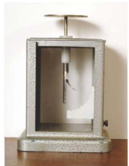
▲ Figure 4 The charged gold leaf electroscope
