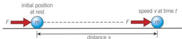
▲ Figure 1 Gaining kinetic energy
