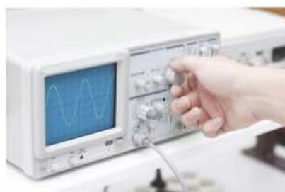
▲ Figure 1 Using a cathode ray oscilloscope (CRO) to give a voltage–time graph of a wave
