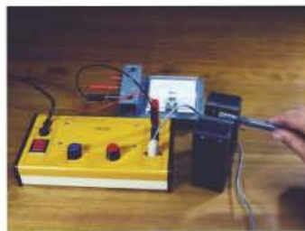
▲ Figure 4 Using a Hall probe
