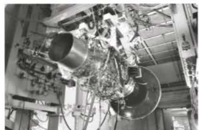
▲ Figure 2 Measuring engine wear
