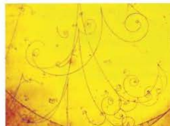
▲ Figure 2 Charged particles in a magnetic field
