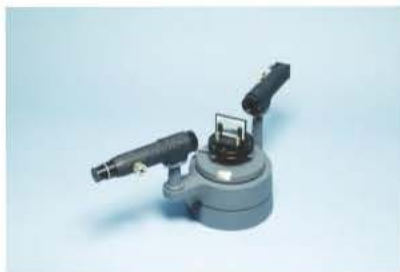
▲ Figure 4 A spectrometer fitted with a diffraction grating
